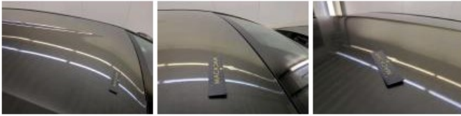
Roof, Hail damage, Paintless dent repair (hail)
