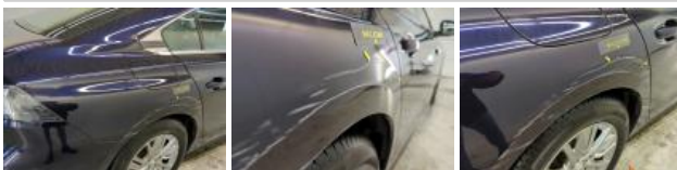
Door RR, Scratch(es), Repair and paint (complete)
