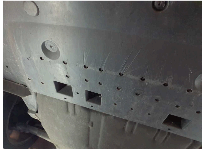
Damage 2: Body: Underbody panelling (+verkratz) - Malposition - Un- / install
