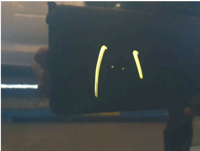
Damage 10: Door - front right side: Door (+delle) - Scratch(es) - Repair and paint
