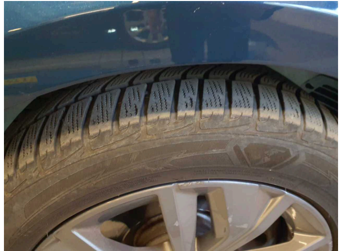
Damage 9: Wheel / tyres: Tyre - front (3mm) - Does not meet the leasing specifications - Replace
