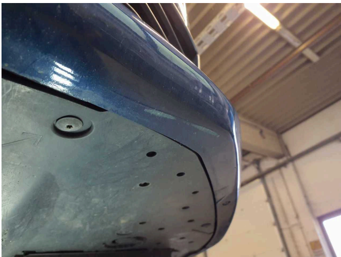
Damage 6: Front bumper: Front bumper (unterhalb) - Scratched - Smart repair
