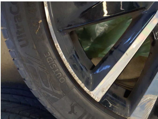
Damage 11: 2nd wheel set: 2 alloy rims - Scratched - Replace
