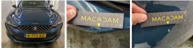
Bonnet, Scratch(es), Repair and paint (complete)
