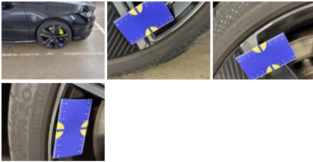
Tyre RR, Worn, Acceptable
