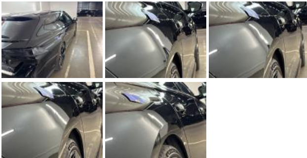
Roof pillar R, Dent(s), Paintless dent repair
