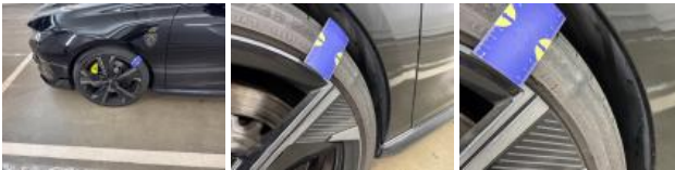
Alloy rim FL polished, Scratch(es), Acceptable
