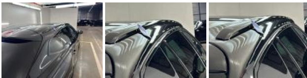
Roof, Deformed / Strained, Repair and paint (complete)
