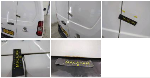
Boot door panel RL, Rust, Repair and paint (complete)
