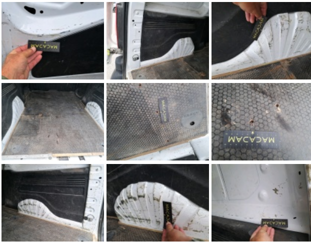
Internal boot lining R, Broken, Replace
