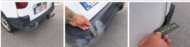
Boot door panel RL, Dent(s) and scratch(es), Acceptable
