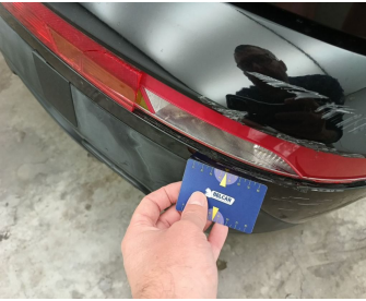
Bumper Rear // Replace & Painting-cracked
