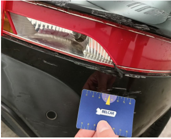
Bumper Rear // Replace & Painting-cracked
