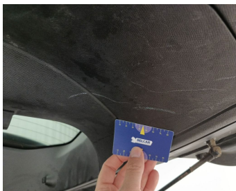
Trunk Lid Interior Coating / Complete Panel / Replace-scratch
