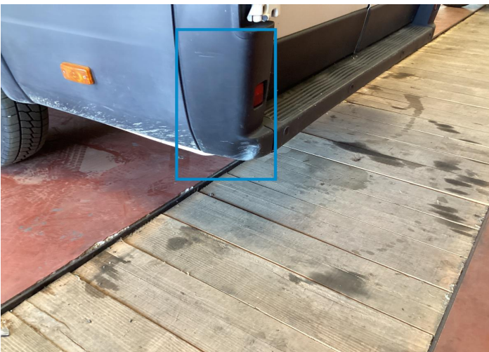
11. Corner Bumper / Back Left Bodywork / Dent / Deformation -
