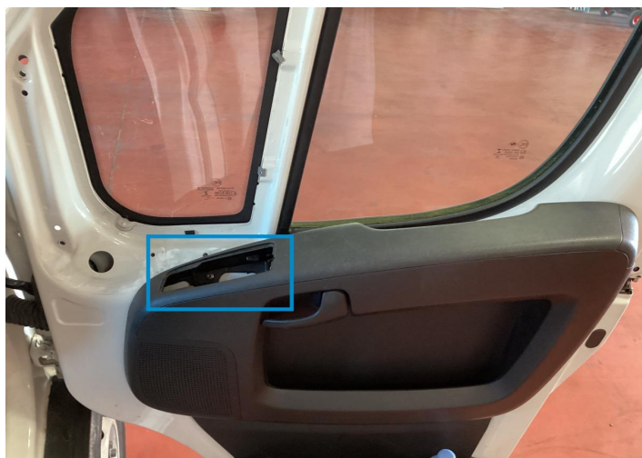
5. Window Switch / Front Right Interior / Missing -
