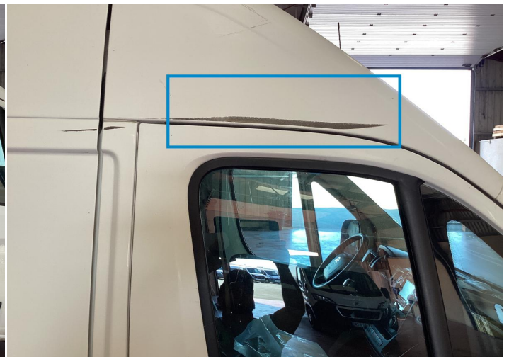
22. Roof Paint / Scratch / Line -
