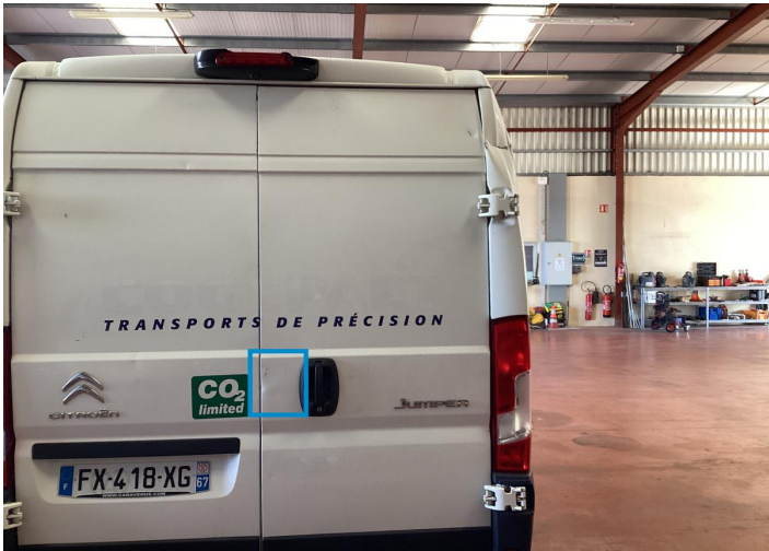
15. Swing Door / Back Right Bodywork / Dent / Deformation -
