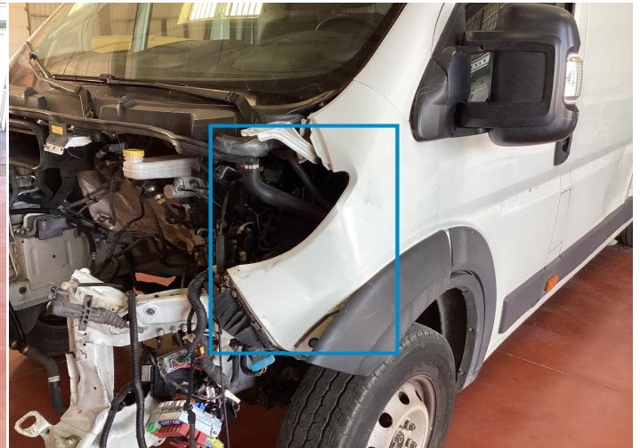
8. Fender / Front Left Bodywork / Dent / Deformation -
