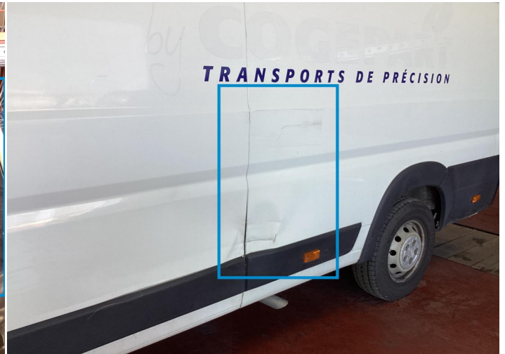
10. Side Panel / Back Left Bodywork / Dent / Deformation -
