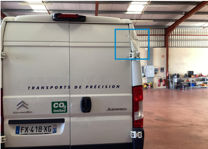
16. Swing Door / Back Right Bodywork / Dent / Deformation -
