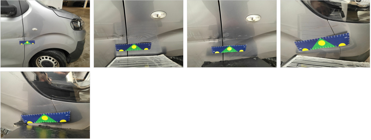
Wing Front right // Repair & Painting: AA - Scratch +Dent
