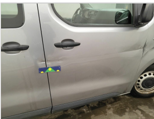
Door Rear Right // Repair & Painting: AA - Scratch +Dent
