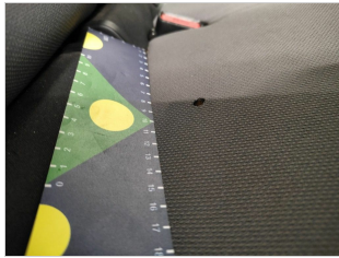
Seat Rear Right / Bottom Coating / Replace: J - Incinerated
