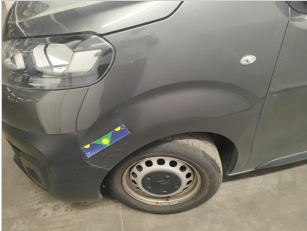
Wing Front Left // Painting: E - Scratch
