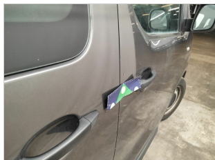
Door Front Right // Smart Repair Small: AA - Scratch +Dent
