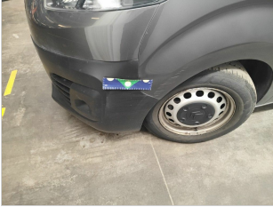
Bumper Front // Replace without painting: E - Scratch
