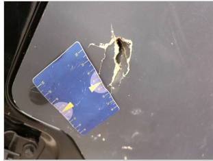
Trunk Lid Interior Coating / MDF Rear Left / Replace: C - Hole
