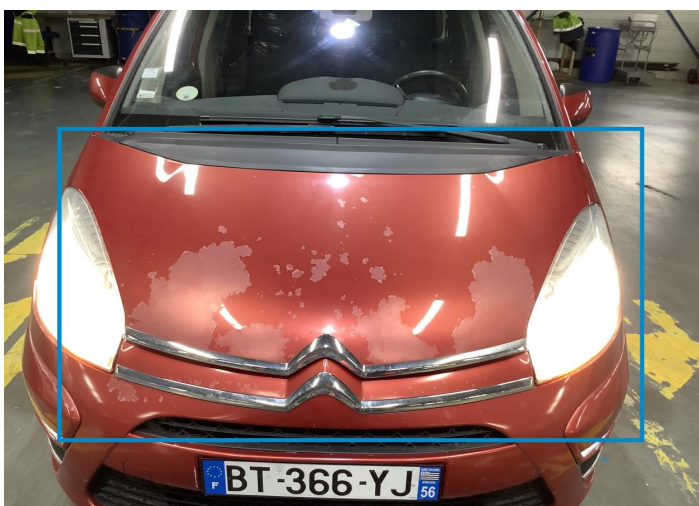
33. Hood Paint / Poor Previous Repair -
