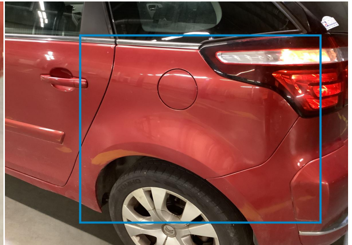
44. Fender / Back Left Paint / Scratch / Line -
