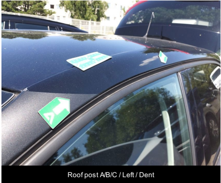
Roof post AB/C / Left / Dent
