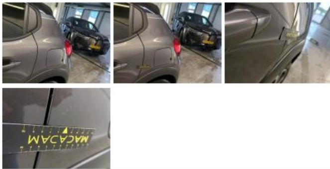
Door RL, Scratch(es), Repair and paint (complete)
