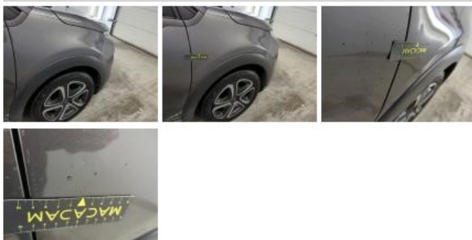
Wing RR, Dent(s), Repair and paint (complete)
