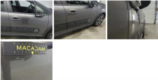
Door RR, Scratch(es), Repair and paint (complete)
