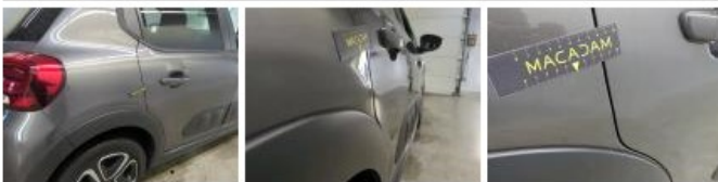
Roof pillar R, Scratch(es), Repair and paint (complete)
