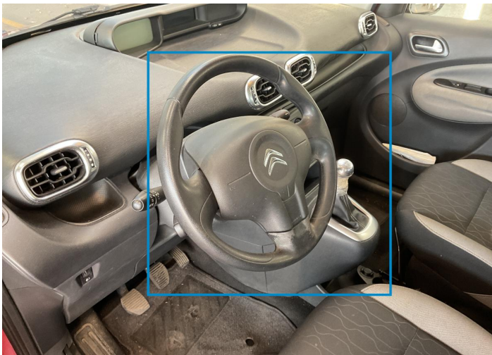
9. Steering Wheel / Front Interior / Worn - out -
