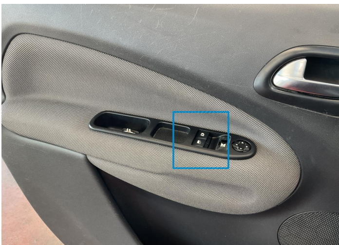
30. Window Switch / Front Left Interior / Dysfunctional -
