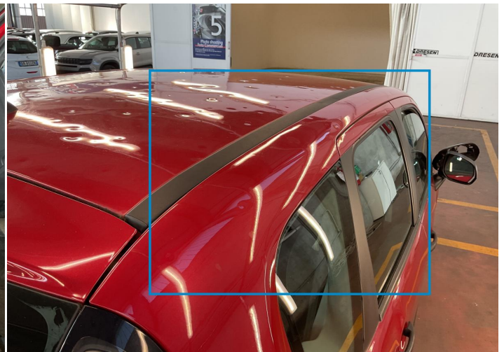
8. Pillar / Front Right Bodywork / Dent / Hail Area -
