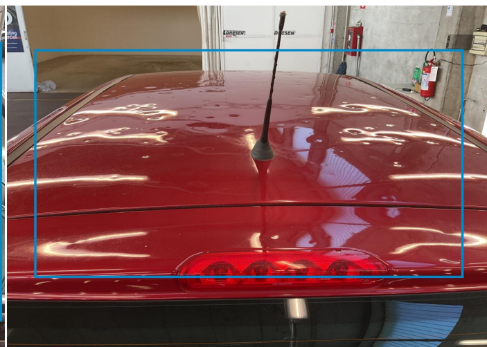
2. Roof Bodywork / Dent / Hail Area -
