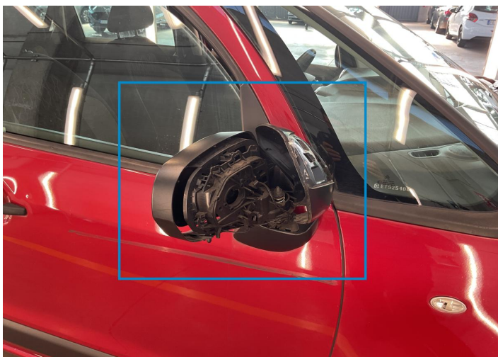
15. Mirror Shell / Front Right Bodywork / Breakage -
