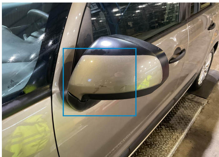
11. Mirror Shell / Front Left Bodywork / Breakage -
