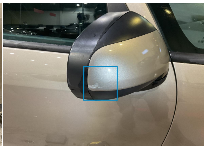
6. Mirror Shell / Front Right Paint / Chipping -
