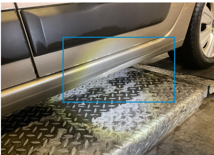
12. Rocker Panel / Center Left Bodywork / Dent / Deformation -
