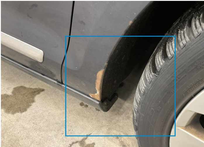
13. Fender / Front Right Paint / Corrosion -
