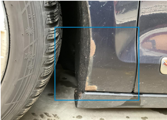
3. Fender / Front Left Paint / Corrosion -
