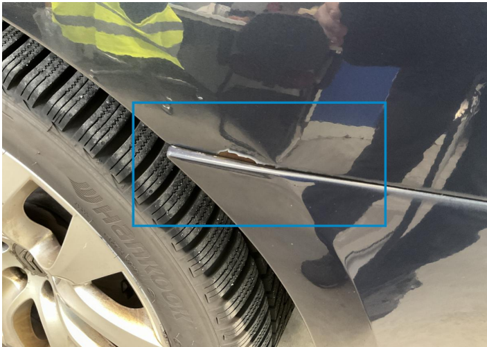
7. Side Panel / Back Left Paint / Corrosion -
