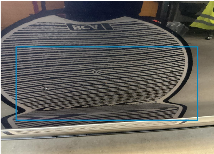
4. Door / Front Left Bodywork / Dent / Dent -
