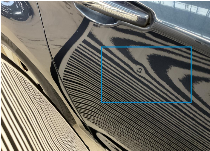
11. Door / Back Right Bodywork / Dent / Dent -
