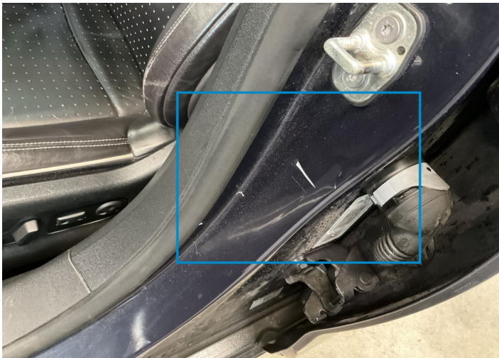
5. Pillar / Front Left Bodywork / Dent / Dent -
