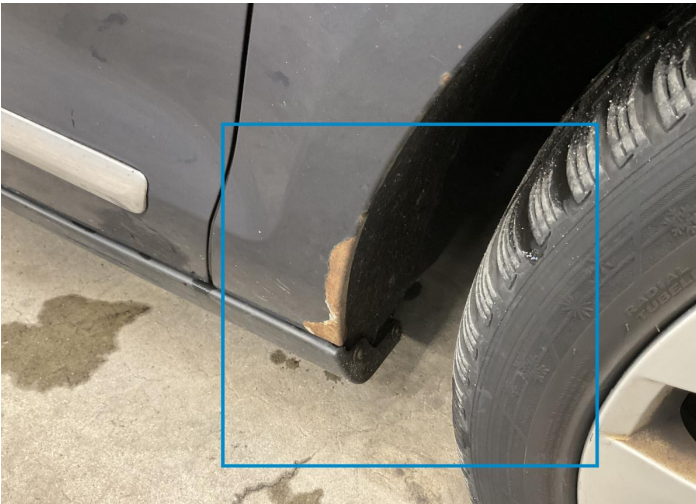
13. Fender / Front Right Paint / Corrosion -
