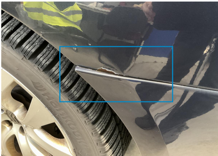
7. Side Panel / Back Left Paint / Corrosion -
