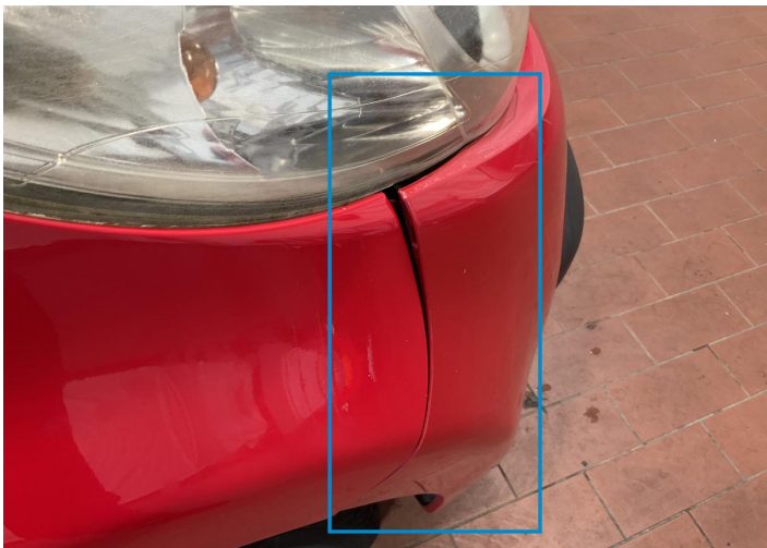
1. Bumper / Front Bodywork / Breakage / Crack -
