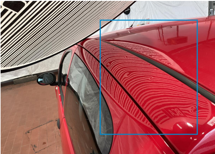
4. Side Panel / Back Left Bodywork / Dent / Hail Area -
