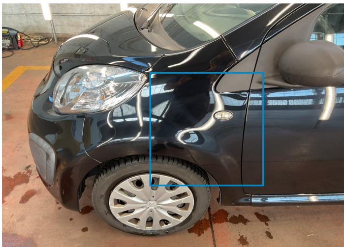
9. Fender / Front Left Paint / Scratch / Line -
