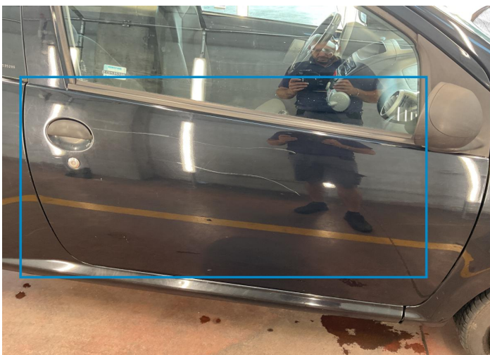
18. Door / Front Right Paint / Scratch / Line -
