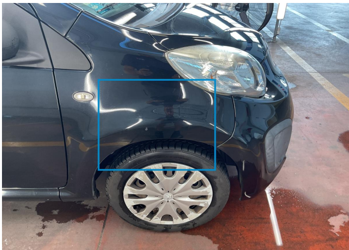
5. Fender / Front Right Paint / Poor Previous Repair -
