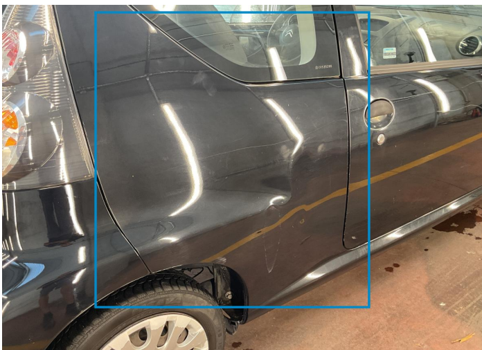
16. Fender / Back Right Bodywork / Dent -
