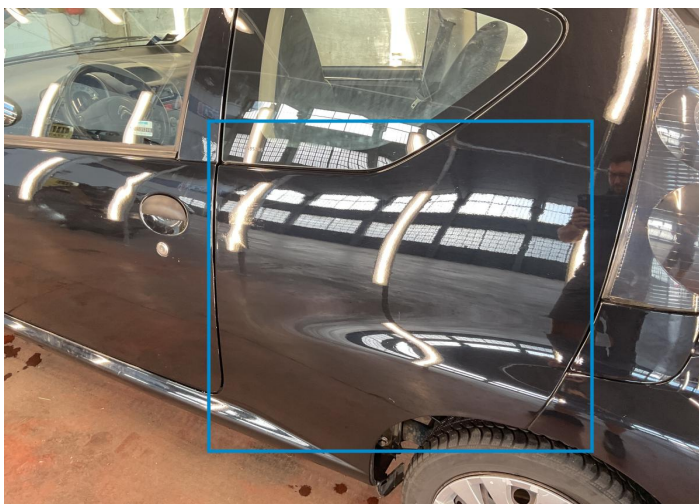
11. Fender / Back Left Bodywork / Dent / Hail Area -
