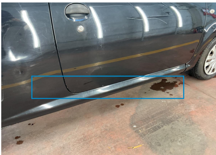
17. Rocker Panel / Center Right Bodywork / Dent -
