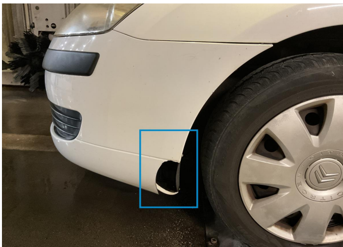
3. Corner Bumper / Front Left Bodywork / Breakage / Crack -
