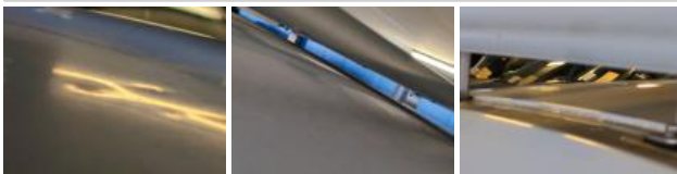
Roof, Dent(s), Paintless dent repair
