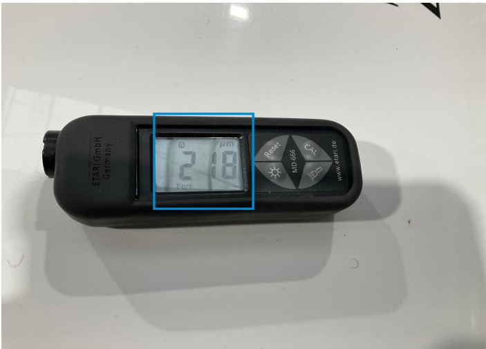
18. Hood Paint / Poor Previous Repair -
