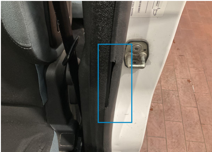
15. Door Joint / Front Left Middle Bodywork / Breakage / Crack -
