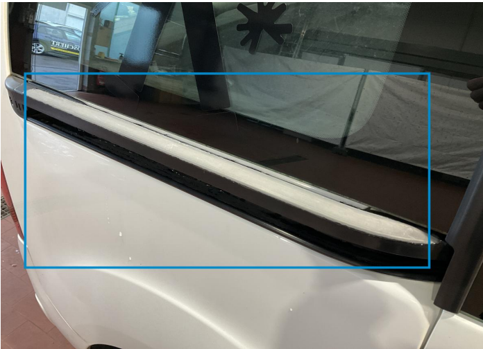
19. Door Slide / Right Paint / Poor Previous Repair -
