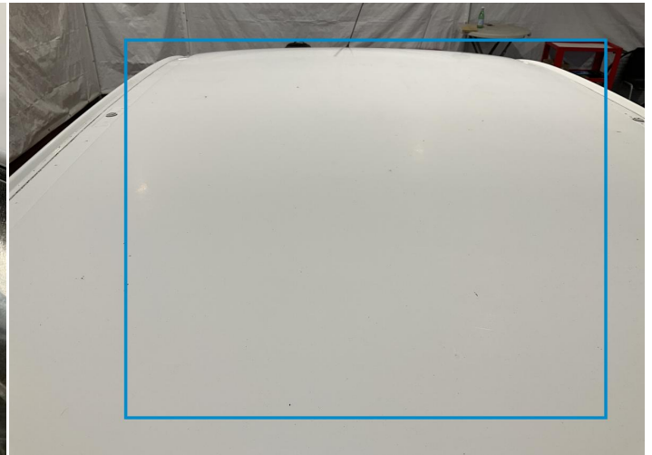
22. Roof Paint / Poor Previous Repair -
