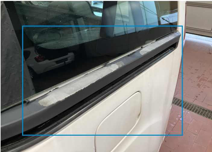
16. Door Slide / Left Paint / Poor Previous Repair -
