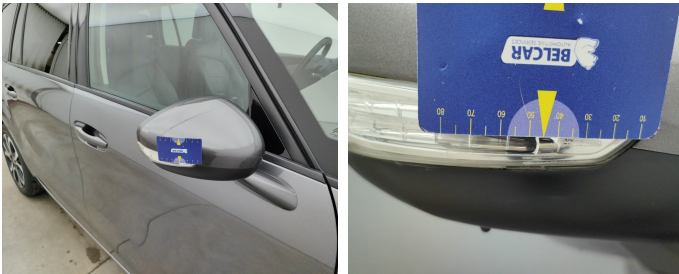
Side View Mirror Right / Direction Indicator / Replace-scratch
