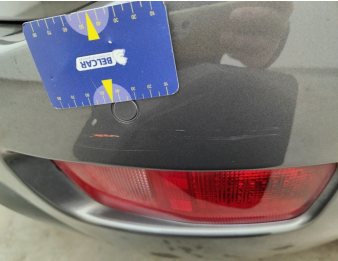
Bumper Rear // Painting-scratch
