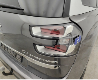
Light / Rear Right On Rear Bonnet / Replace-scratch
