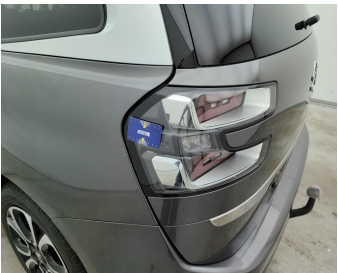
Light / Rear Left On Rear Bonnet / Replace-scratch
