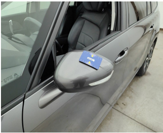
Side View Mirror Left // Painting-scratch
