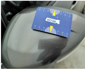
Side View Mirror Left // Painting-scratch
