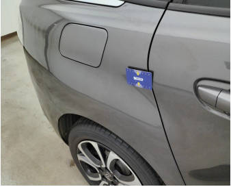
Wing Rear Right // Polish-scratch
