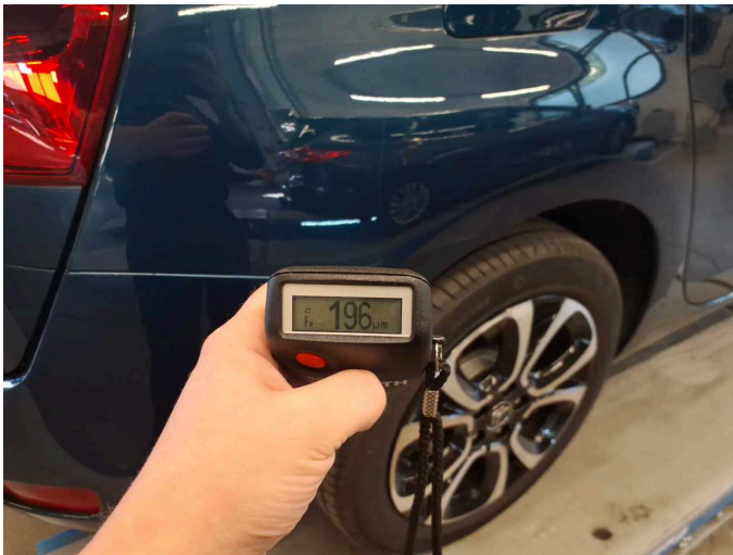
Repainting 1: Bonnet, Side panel - rear left side, Side panel - rear right side, Door - rear left side, Door - rear right side
