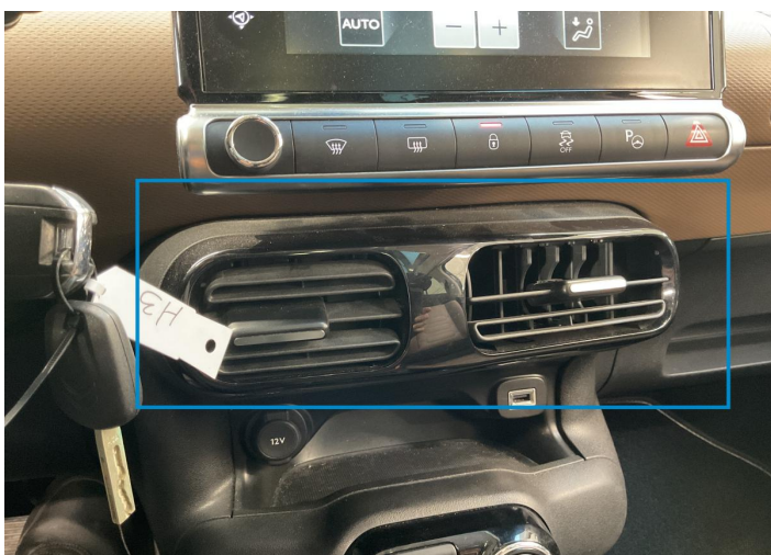
9. Aeration Grid / Front Center Interior / Broken -
