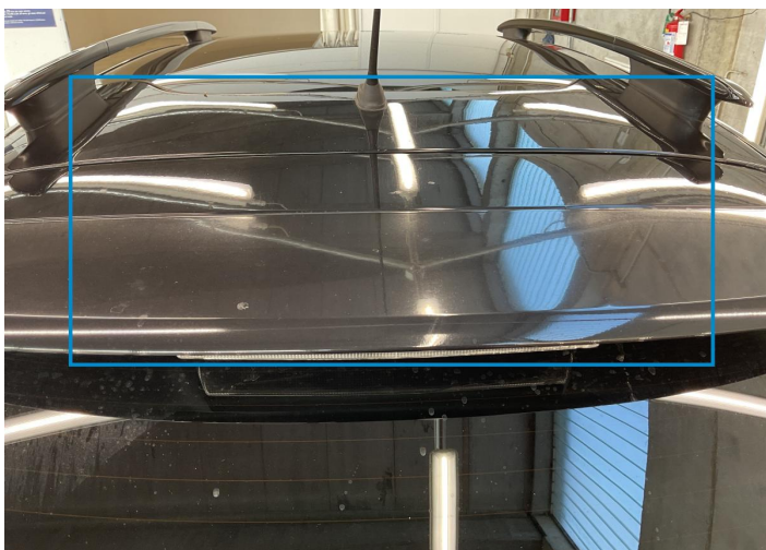
7. Roof Bodywork / Dent / Hail Area -
