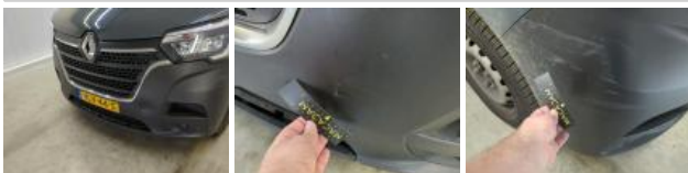
Bumper grille, Deformed / Strained, Replace
