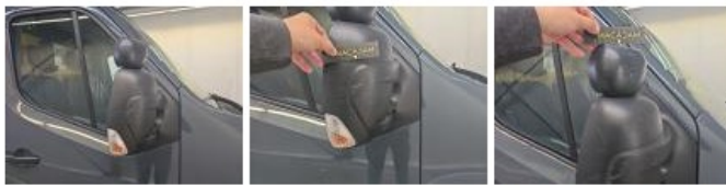
Mirror side repeater R, Scratch(es), Replace
