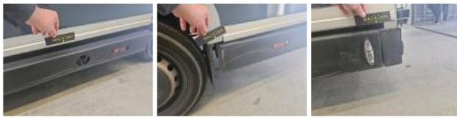
Bumper F, Dent(s) and scratch(es), Replace
