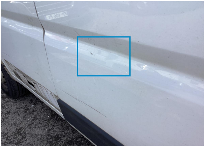
11. Door / Back Right Bodywork / Dent / Dent -
