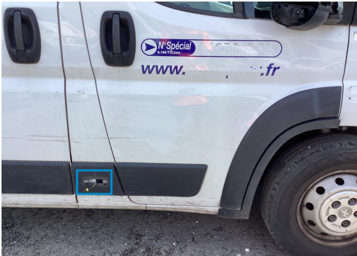
9. Door / Front Right Missing Part -
