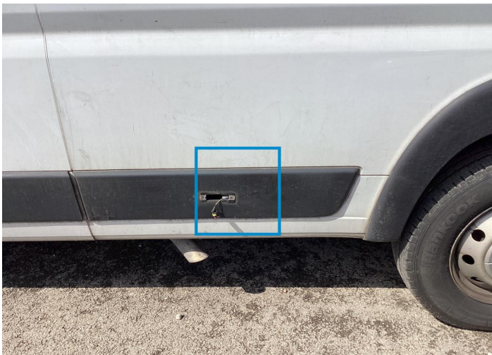
19. Wing Stick / Back Left Missing Part -
