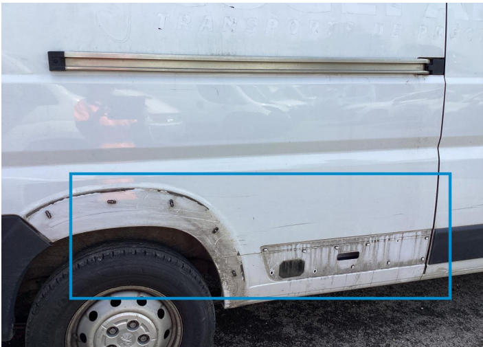
12. Wing Stick / Back Right Missing Part -
