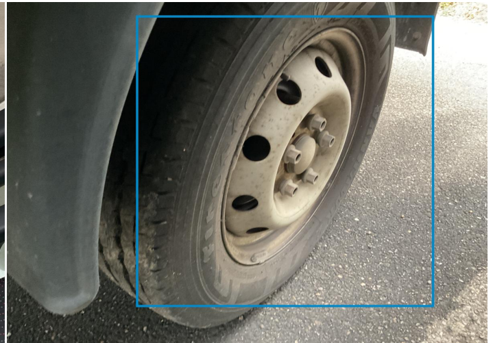
2. Rim / Back Left Out of Bodywork / Scratch -
