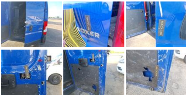
Internal boot lining R, Broken, Replace
