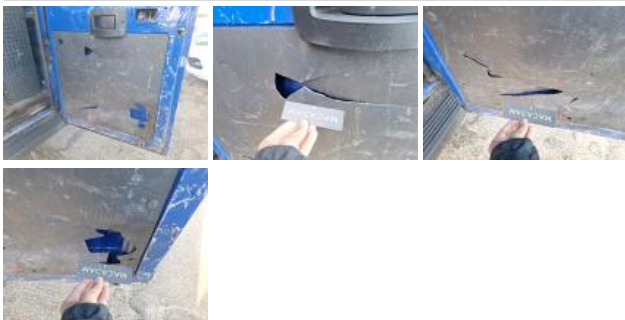
Internal boot lining R, Broken, Replace
