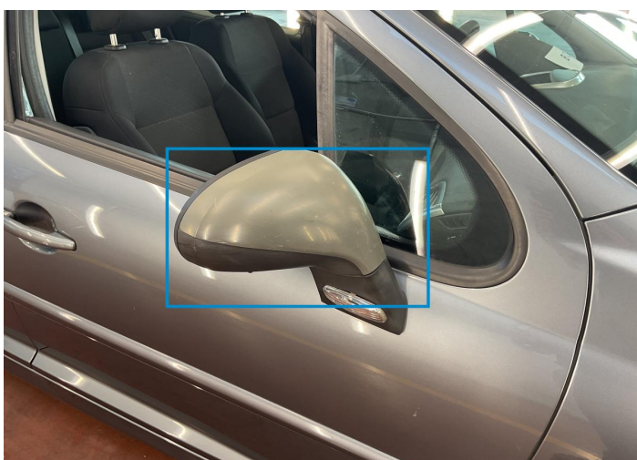
23. Mirror Shell / Front Right Paint / Scratch / Line -
