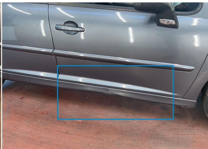
12. Rocker Panel / Center Right Bodywork / Dent -
