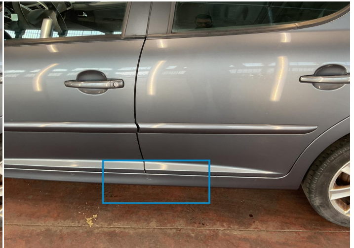
26. Rocker Panel / Center Left Bodywork / Dent -
