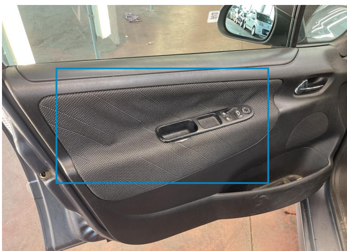
9. Panel Filling / Front Left Interior / Broken -
