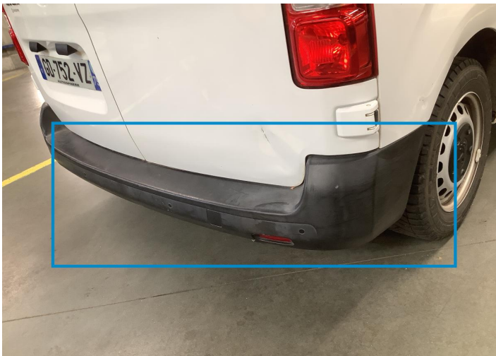
27. Shield / Back Paint / Scratch / Line -
