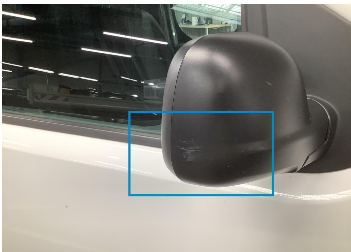
13. Mirror / Front Right Paint / Scratch / Line -
