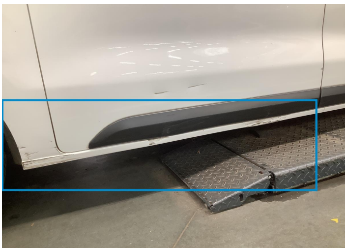
17. Rocker Panel / Center Right Bodywork / Dent / Dent -
