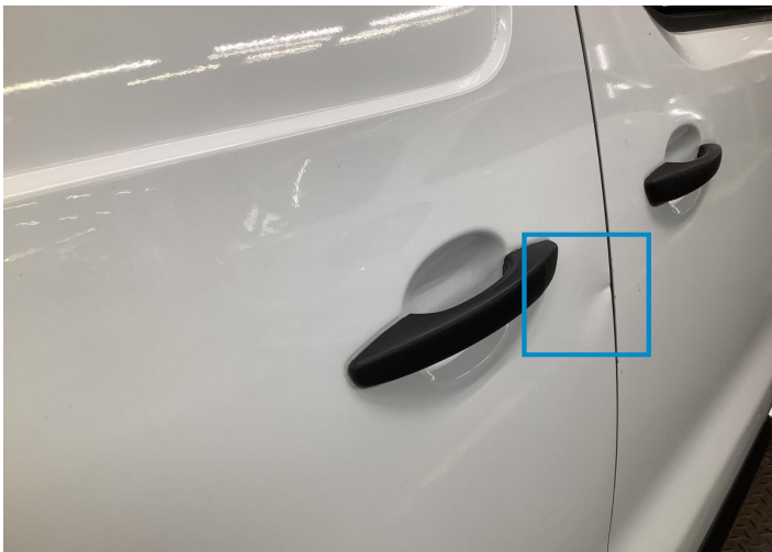
25. Door / Back Right Bodywork / Dent / Dent -
