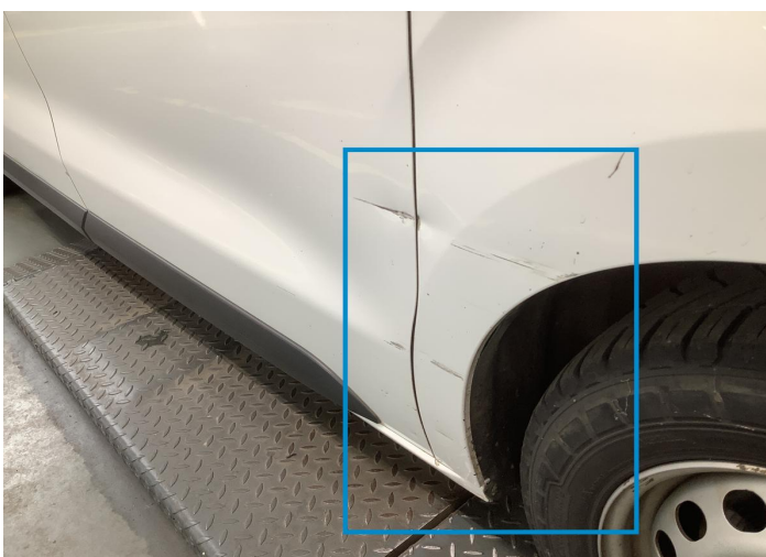
10. Fender / Front Right Bodywork / Dent / Dent -
