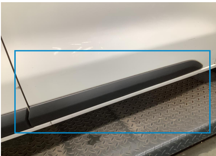
16. Door Side Molding / Front Right Paint / Scratch / Line -
