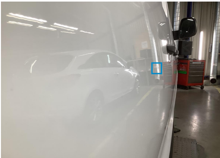
26. Door / Back Right Bodywork / Dent / Dent -
