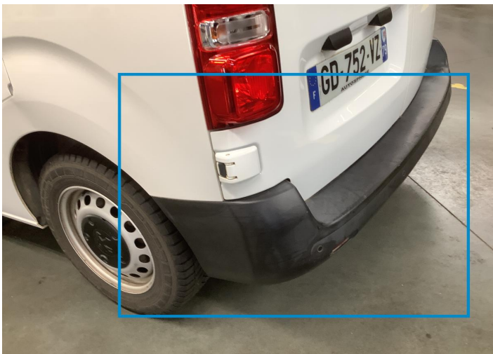
30. Shield / Back Paint / Scratch / Line -
