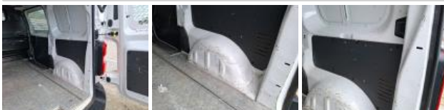
Internal boot lining R, Scratch(es), Acceptable
