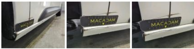
Wing FL, Scratch(es), Repair and paint (complete)
