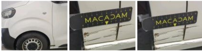
Door FL, Scratch(es), Repair and paint (complete)
