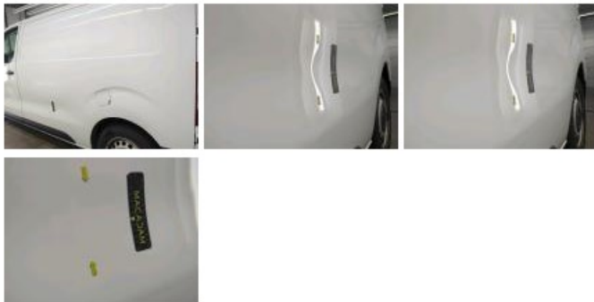
Door FR, Scratch(es), Repair and paint (complete)
