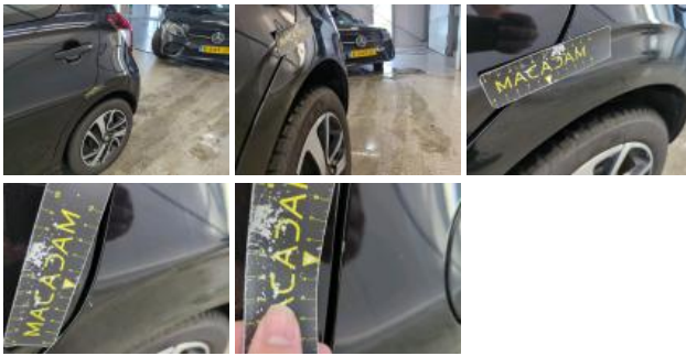
Door FL, Bad repair, Repair and paint (complete)
