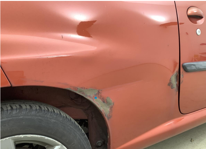
13. Side Panel / Back Right Paint / Corrosion -
