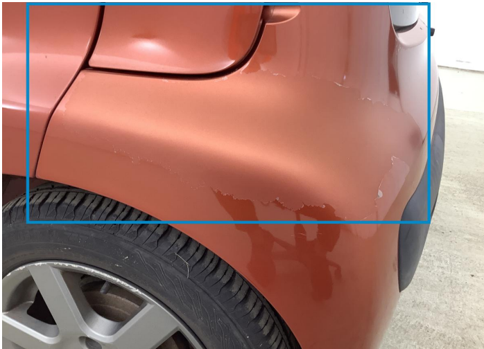
1. Bumper / Back Bodywork / Dent / Deformation -
