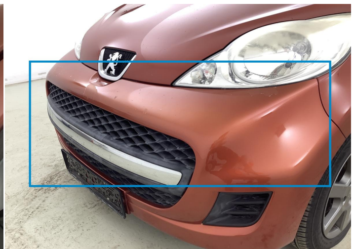
6. Bumper / Front Bodywork / Dent / Deformation -
