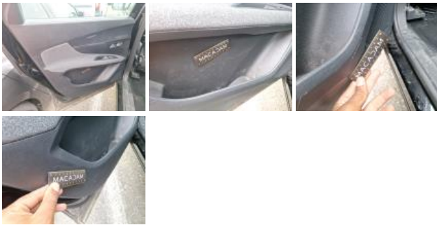
Inner door sill RL, Dent(s) and scratch(es), Repair and paint (complete)
