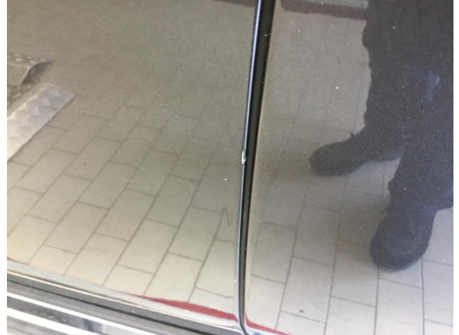
Tür vorne links - Rostansatz - smart Repair
