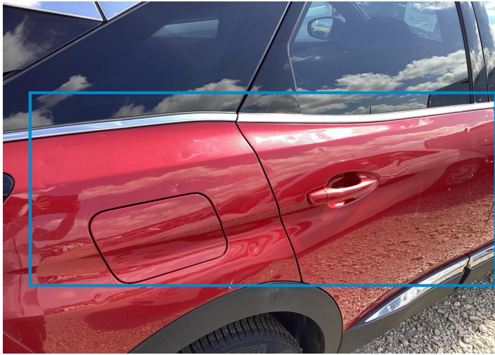
5. Fender / Back Right Bodywork / Dent / Hail Area -
