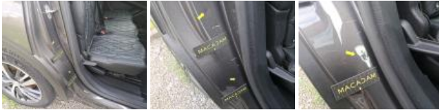
Door RR, Dent(s), Spot repair
