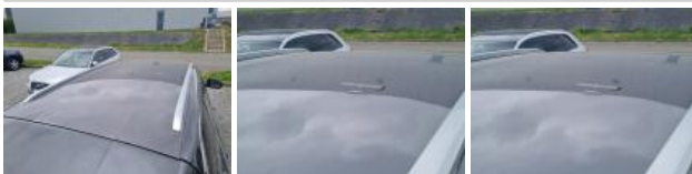
Roof, Dent(s), Paintless dent repair
