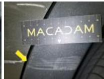
Wing RL, Dent(s) and scratch(es), Repair and paint (complete)
