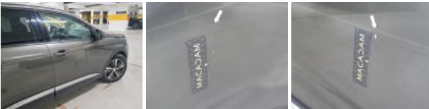
Mirror side repeater R, Scratch(es), Replace
