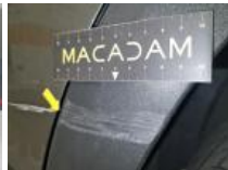
Wing RL, Dent(s) and scratch(es), Repair and paint (complete)
