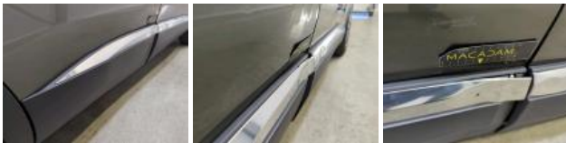
Door trim FR, Deformed / Strained, Replace
