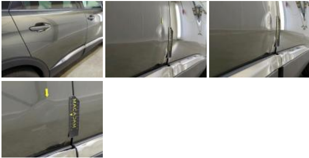
Door trim RR, Deformed / Strained, Replace
