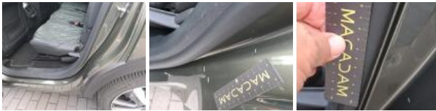
Door RL, Dent(s), Repair and paint (complete)
