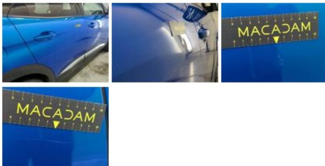
Door FR, Scratch(es), Repair and paint (complete)
