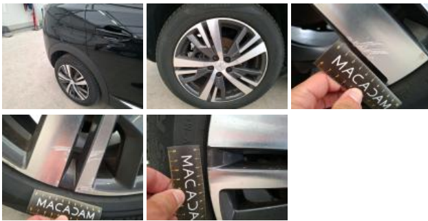
Tyre RR, Tear, Replace
