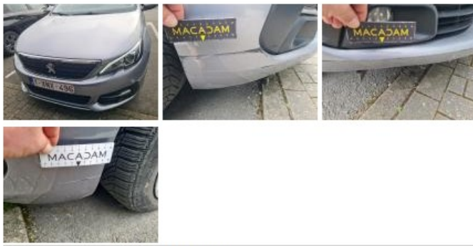
Bumper moulding F, Scratch(es), Replace
